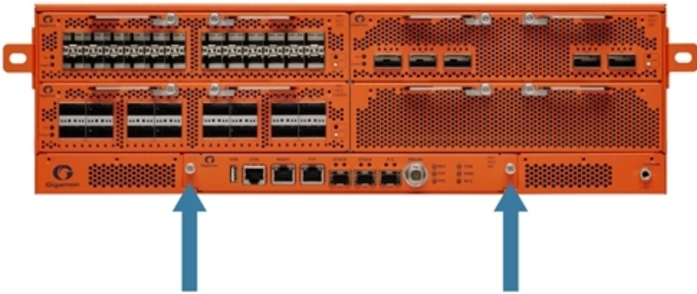
Figure 15 Extension Board Screw Location on GigaVUE-HC3 Front
